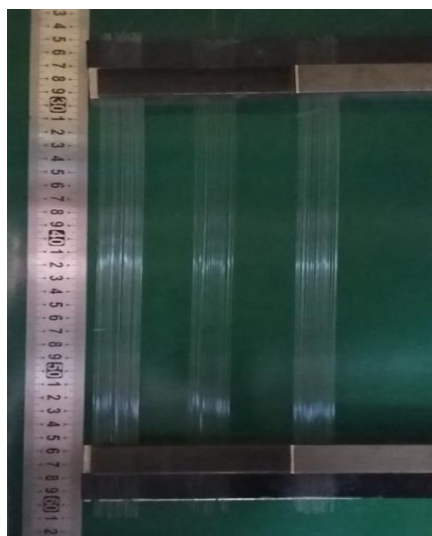
Fig. 3 Locating HGFs at angle of 0° in the fixture
