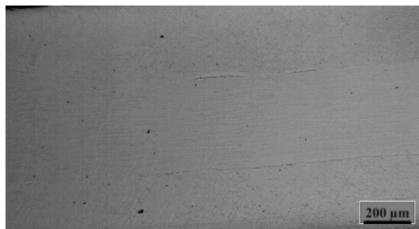
Fig 5 microstructure of primary sandwich of multi-layered Al/Brass composite
