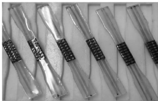
Fig. 20 Specimens of self-healable glass fibers- epoxy composite containing 3D microvascular network [64]
