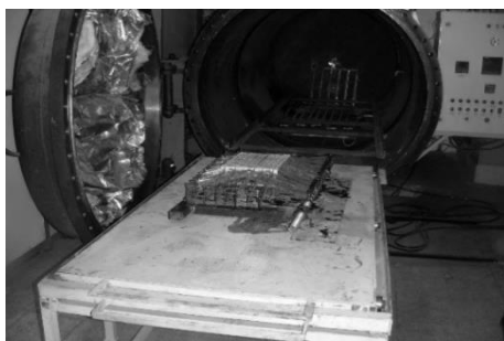
Fig. 2. Curing grid stiffened core in autoclave
