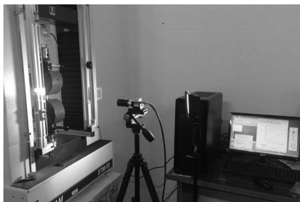
Fig 4 A set up of tensile test with DIC equipment's
