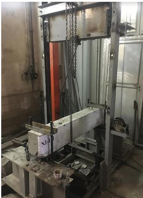
Fig. 9 Impact loading test setup
