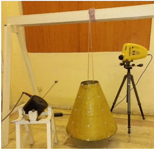
Fig. 4 The experimental setup and equipment for modal test of anisogrid composite lattice conical shell
