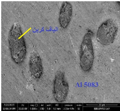
Fig. 16 SEM Image of the Interface Region in Al 5083-4% vol C sf Sample
