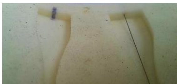
Fig. 5 The location of NiTi wire in the mold of latex samples
