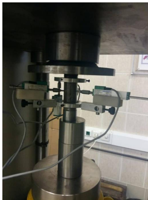
Fig. 2 Uniaxial stress device with integrated sensors to measure lateral displacement
