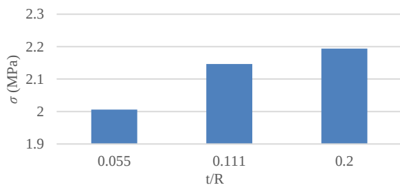
Fig. 24 The effect of capsule thickness ratio on the ultimate fracture stress in a two-wire sample
