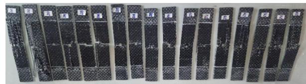
Figure 31 Broken specimens of tensile and fatigue after testing
