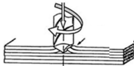
Fig. 5 Delamination at the entrance of the drill [3]
