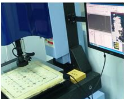
Fig. 3 Measurement of diameter with three points around the hole by VMM
