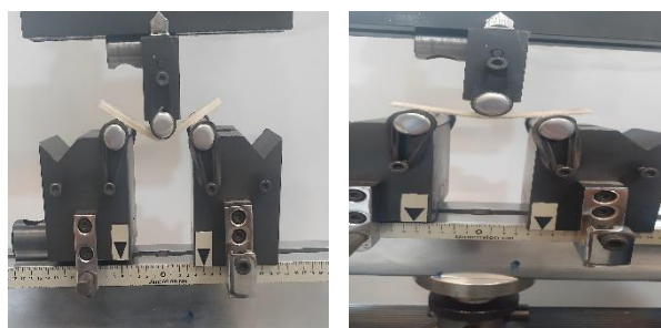
Fig. 7 Photographs of the specimens after the flexural test: a) [F_2/I_2]_s , b) [I_2/F_2]_s .
