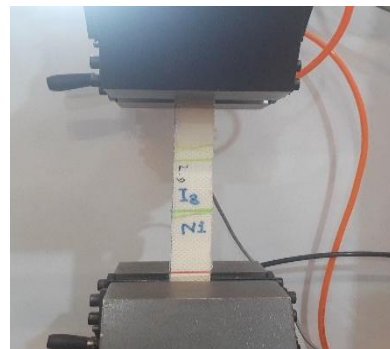
Fig. 2 View of the STM-150 universal testing machine and the configuration of the composite specimen during the uniaxial tensile test.
