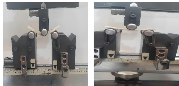
Fig. 7 Photographs of the specimens after the flexural test: a) [F_2/I_2]_s , b) [I_2/F_2]_s .
