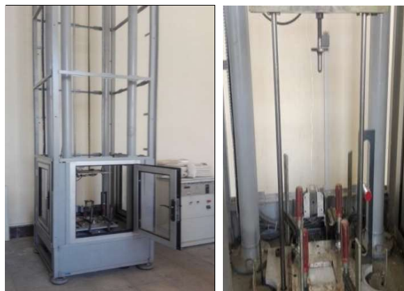
Fig. 3 Drop-weight impact testing machine
