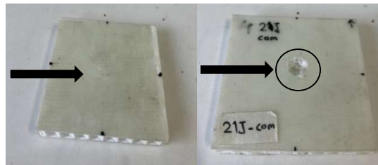
Fig. 14 Front and back surfaces of PLA/Glass specimen after low-velocity impact at 21 J
