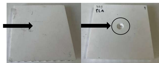
Fig. 12 Failure mechanisms and experimental surfaces of pure PLA specimen under 10 J impact energy
