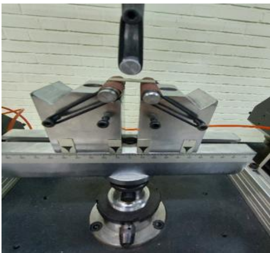
Fig. 5 Devices and equipment used to perform the ILSS test
