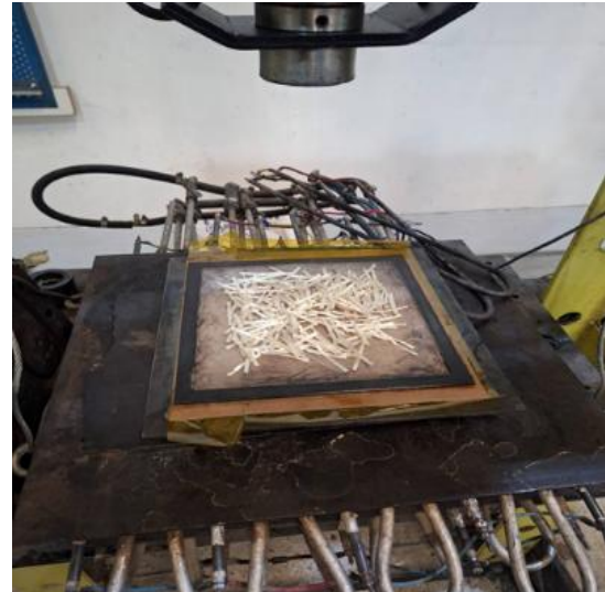
Fig. 2 Image of a frame containing chopped fibers for producing sheets with a random arrangement
