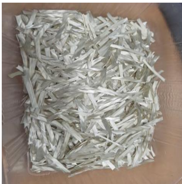
Fig. 1 Image of fibers cut to 2.5 cm in length
