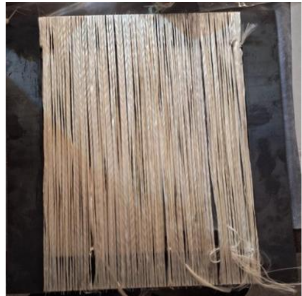
Fig. 3 Image of a frame containing unidirectional fibers for sheet production
