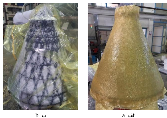
Fig. 3 (a) The Kevlar inner skin and (b) vacuum process of anisogrid composite lattice core
