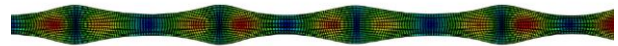
Fig. 10 Propagation of S_0 Lamb wave mode with the frequency of 200 kHz in the intact glass/epoxy composite specimen with the stacking sequence of [0_4/90_4]_s
