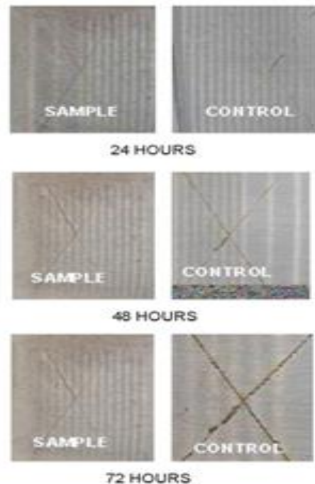
Fig. 3 Self-healing performance of samples after different times of salt spray test [25].
