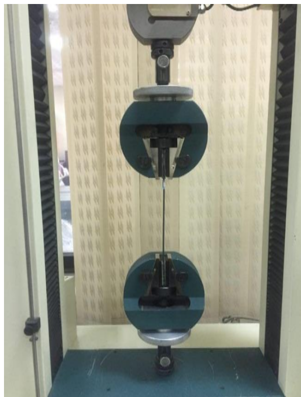
Fig. 1 Nanocomposite specimen in the tensile test device
