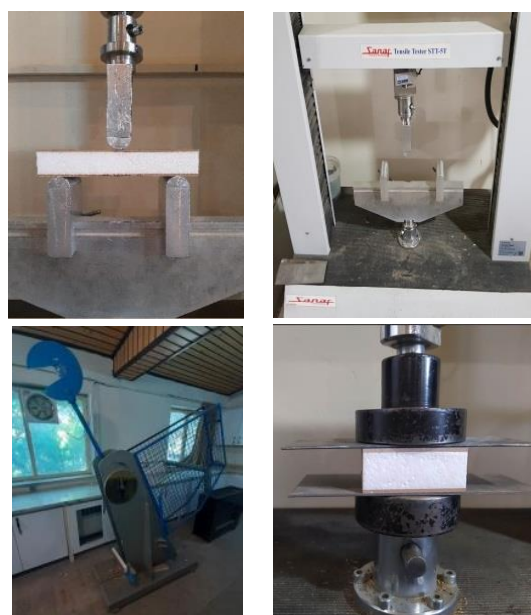
Fig. 3 Methods of performing mechanical tests (mechanical testing machine, bending strength test, compressive strength test, and impact strength test)
