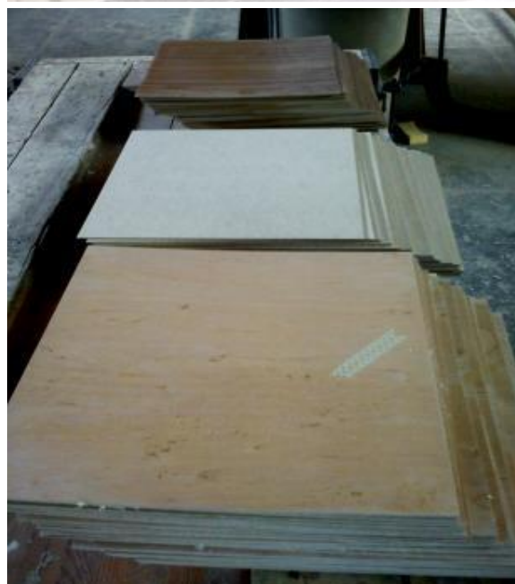
Fig. 1 Polystyrene foam and types of 3 mm fiberboard used in the manufacture of sandwich panel
