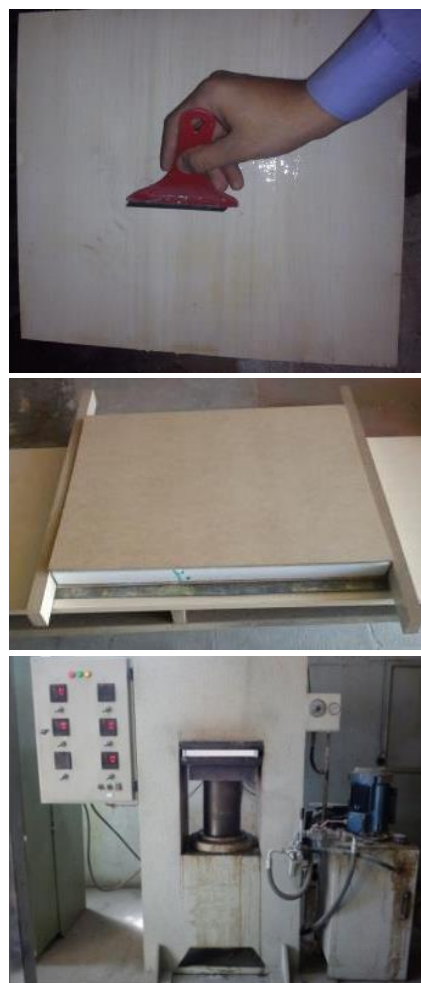
Fig. 2 Gluing, assembly and pressing for the manufacture of sandwich panels
