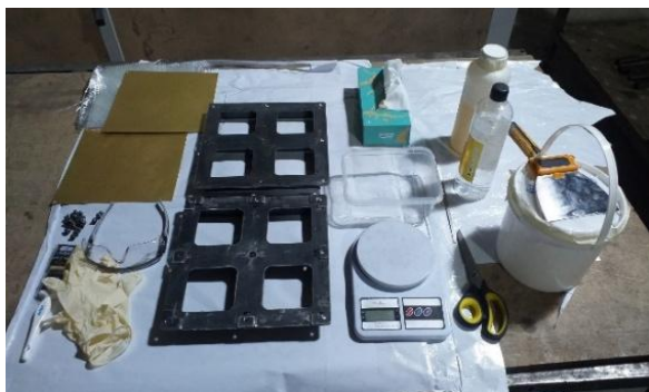
Fig. 3 Tools and materials used for hand lay-up.
