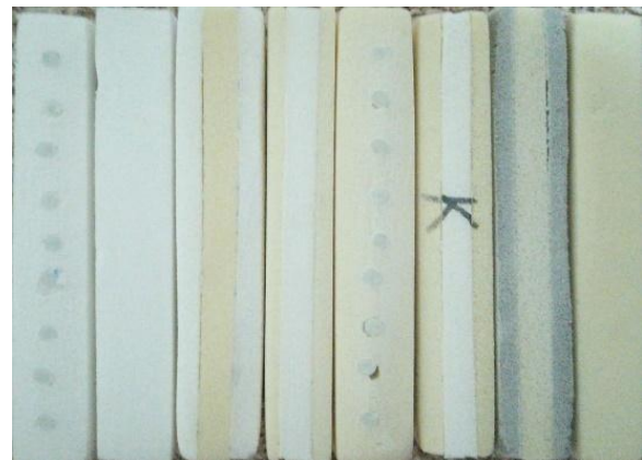
Fig. 3 Top view after face-core bonding
