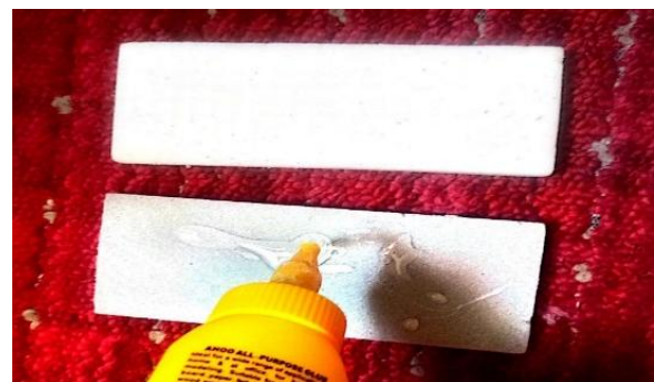
Fig. 2 Preparation of the core for composite fabrication
