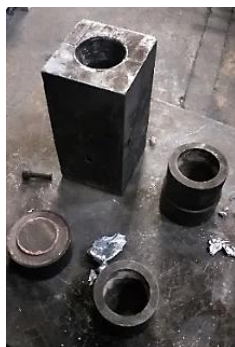
Fig. 2 Casting mold used for in-situ Al-15%Mg 2 Si composite production
