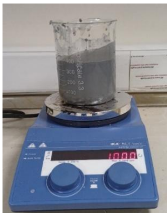
Fig. 2 Stirring the solution with a magnetic stirrer
