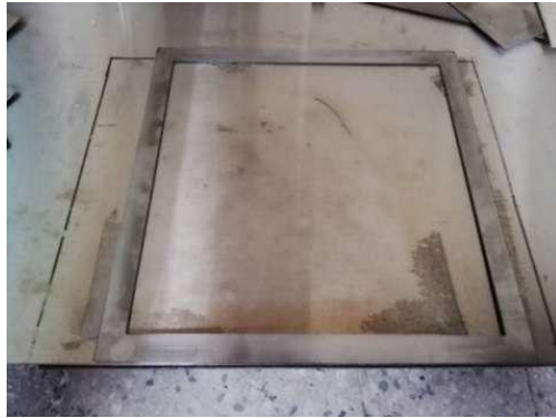
Fig. 3 Metal mold with a thickness of 3 millimeters
