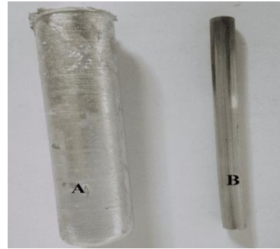
Fig. 2 Image of the AA5083/TiB 2 Composite A) Before Extrusion B) After Hot Extrusion.
