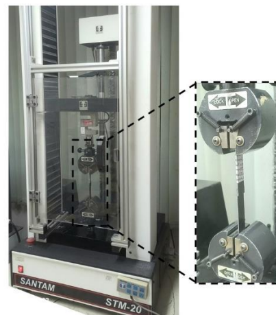
Fig. 5 Lap Shear Strength test with universal testing machine STM-20 on the continuous ultrasonic welding samples.
