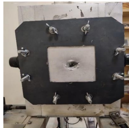
Fig. 10 Clamped specimen in the fixture after testing
