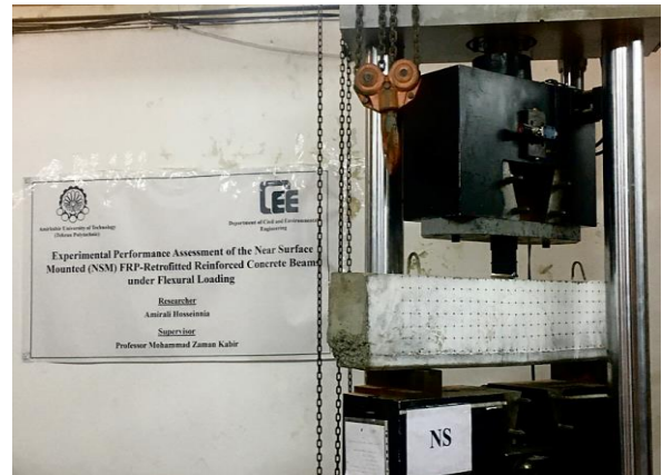
Fig. 6 Test setup for flexural loading
