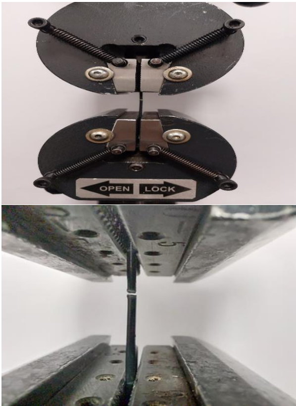
Fig. 2 A sample of the tensile test piece with the device
