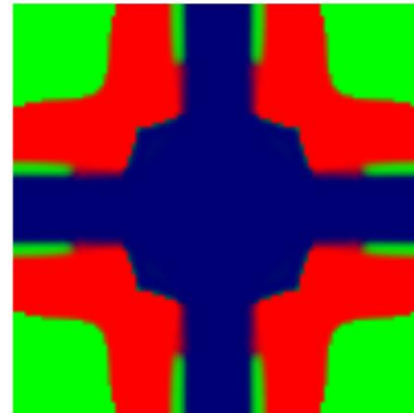
Fig. 13 The designed microstructure with a volume fraction of 0.375 of phase 1 (red) and phase 2 (blue and 0.25 green for the void phase) of solid phases and axial stiffness equal to 0.2889 in two dimensions and 0.3062 in three dimensions
