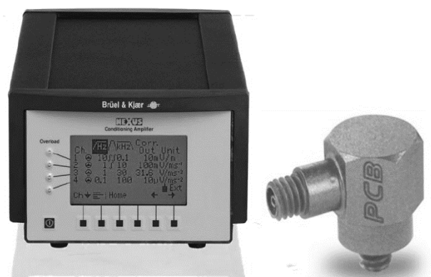
Fig. 6 The accelerator sensor and the amplifier
