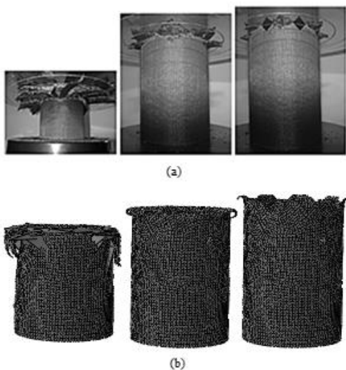
Fig. 5 Collapse behavior of composite crash box: (a) recorded in lab [30], and (b) modelled as shell (with conventional-shell elements)
