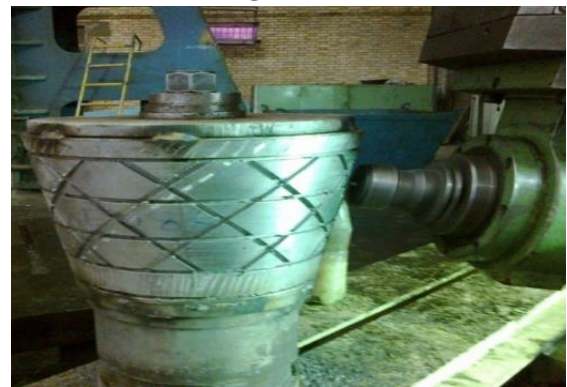
Fig. 2 Metallic mandrel for composite lattice truncated cone
