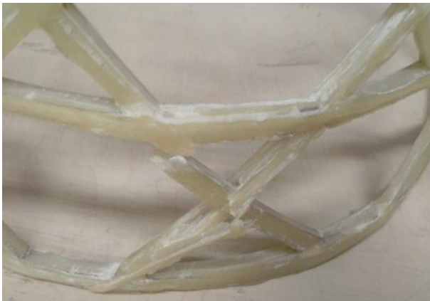
Fig. 8 Local failure mode for composite lattice cone specimen without CNT close to a critical node after axial compressive test
