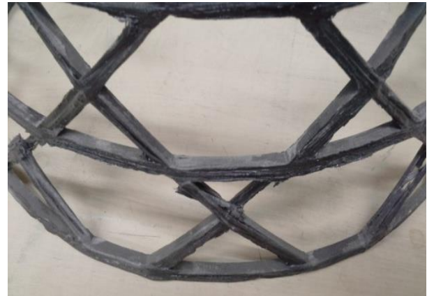
Fig. 11 Local failure mode for composite lattice cone specimen with 2% wt. CNT close to a critical node after axial compressive test
