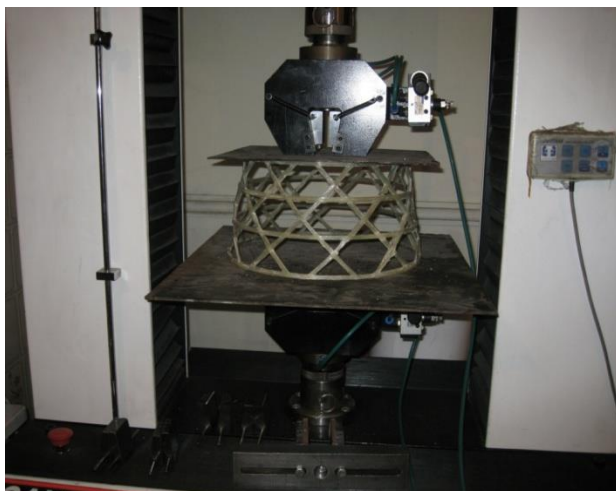
Fig. 4 Axial compression test on the composite lattice truncated cone
