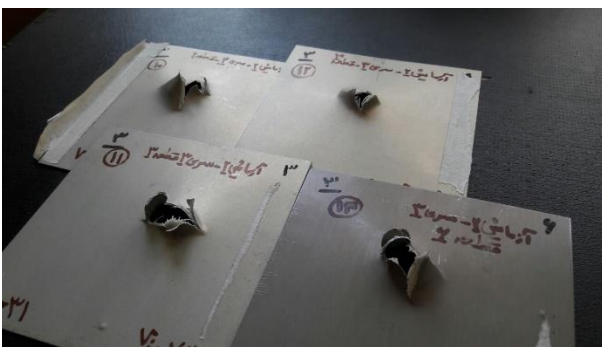
Fig. 9 Sample of FML after impact test
