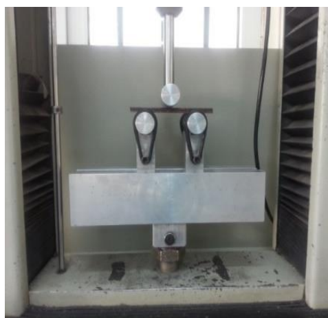
Fig. 5 A specimen under bending test
