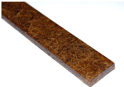
Fig. 3 A specimen of sample A3 for tensile test
