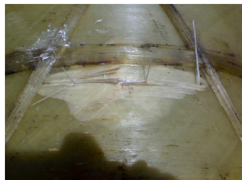
Fig.15 Close-up of the composite after bullet hits its target
