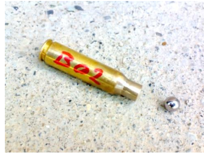
Fig. 7 Picture bullets before insertion into the shell casing
