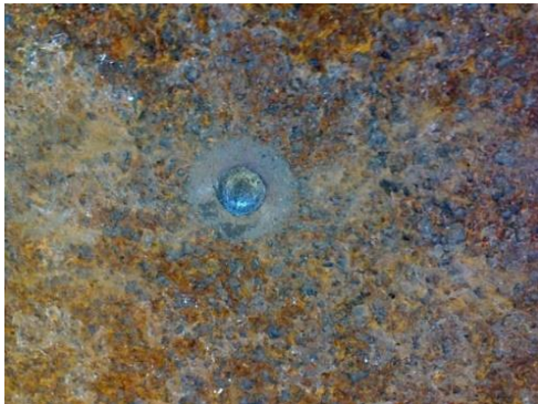
Fig.12 Targets composite image of the back of the goal after hitting the third shot (third test) and bullet impact on its output target
