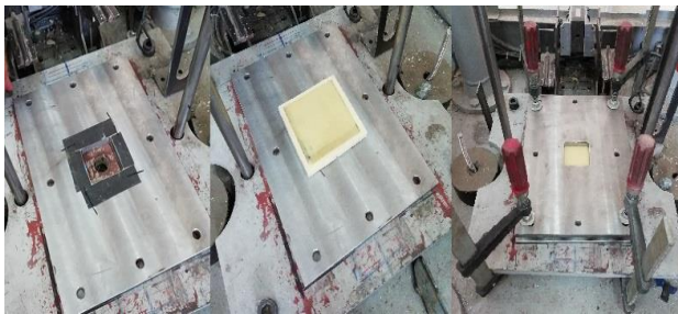
Fig. 6 Fixture of sandwich panel containing Nano silica
