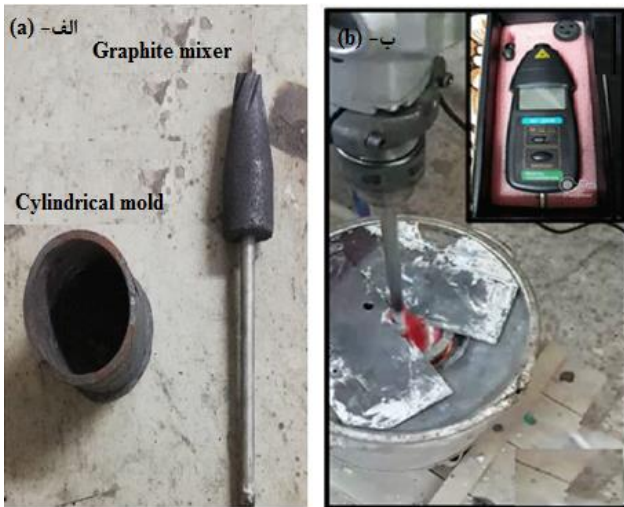
Fig. 2 A: Graphite mixer and cylindrical mold. B: Mixer and power generation setup.
