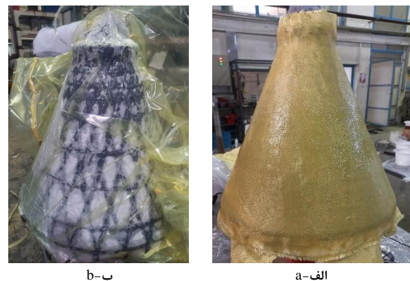
Fig. 3 (a) The Kevlar inner skin and (b) vacuum process of anisogrid composite lattice core
