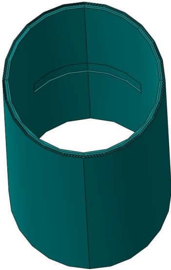
Fig. 6 Partial corrosion in the pipe with a length of 40 mm and a circumferential angle of 90 degrees.
