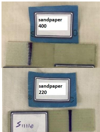
Fig. 17 Two joint samples representing the surfaces sanded by each of the sandpapers
