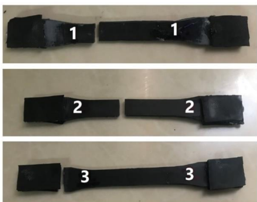
Fig. 33 Dumbbell samples made to check the mechanical properties under the effect of temperature of 80 degrees Celsius
