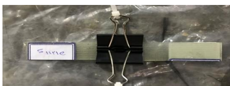
Fig. 22 Adhesive joint sample after applying adhesive and exposure to thickness control constraints
