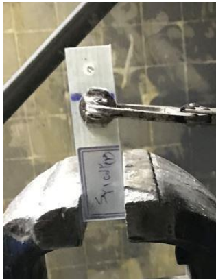
Fig. 26 The sample fixed on the perforated mold after the drilling process
