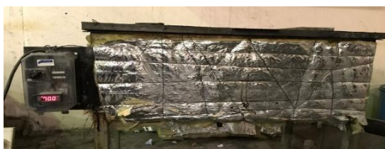
Fig. 23 Placing adhesive joint samples to perform adhesive post-baking
