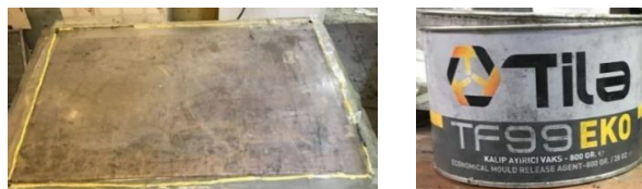
Fig. 7 Separating wax and waxed mold surface
