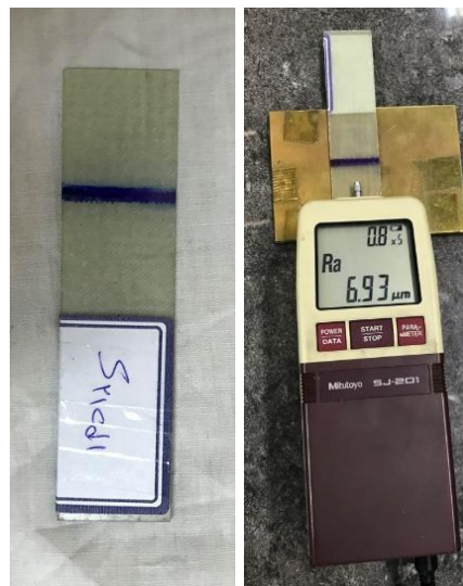
Fig. 19 The unsanded sample and the roughness meter after measuring the Ra parameter
