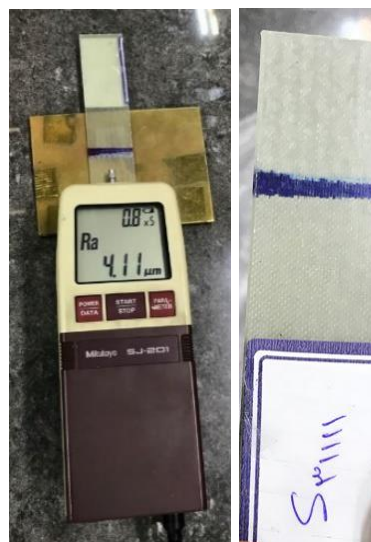
Fig. 20 The sample was sanded with a 220 sander and a roughness meter after measuring the Ra parameter
