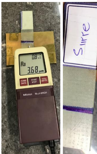
Fig. 21 The sample was sanded with a 400 sander and a roughness meter after measuring the Ra parameter
