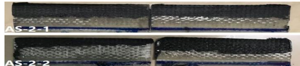
Fig. 58 The surface of adhesive joints based on the zigzag arrangement of four rivets under the effect of temperature of 80 °C after failure
