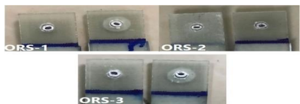
Fig. 48 Optimum surface of rivet joints under the effect of temperature of 80°C after failure
