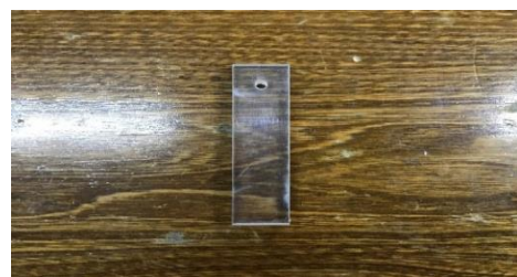
Fig. 25 10 mm thick plexiglass mold with a 5 mm diameter hole
