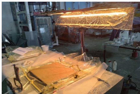
Fig. 6 Curing resin at T=70^{\circ}\text{C} using electrical heater
