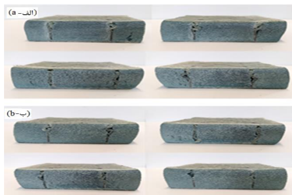
Fig. 18 Deformation of the sample with resin lattice under through thickness compression, (a) four sides of the first samples and (b) four sides of the second sample
