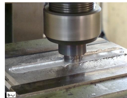
Fig 4 (a) Covering the groove using tool number one and (b) performing the process with multiple passes using tool number two.
