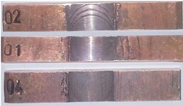
Fig. 3 FSP on parts with codes 01, 02 and 04.
