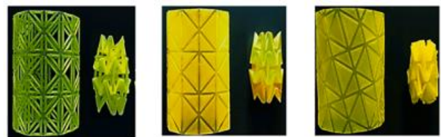
Fig. 19 4D printed stents before and after folding [82]
