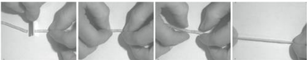
Fig. 5 Self-healing rubber composite at room temperature. The sequence of images from left to right shows cutting, connecting, repairing and stretching the tire after healing [87]
