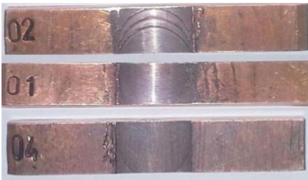
Fig. 3 FSP on parts with codes 01, 02 and 04.
