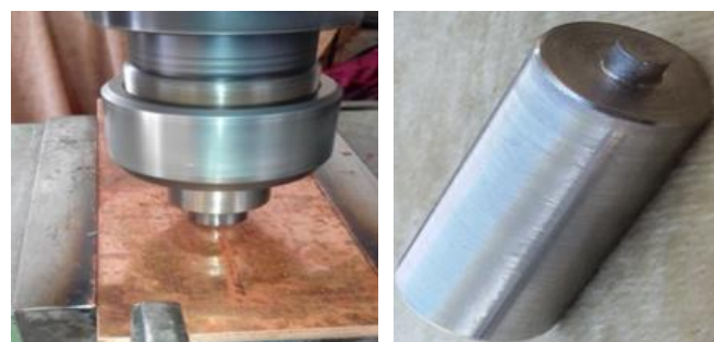
Fig. 2 The tool used and its interaction with the part in the friction stir processing.
