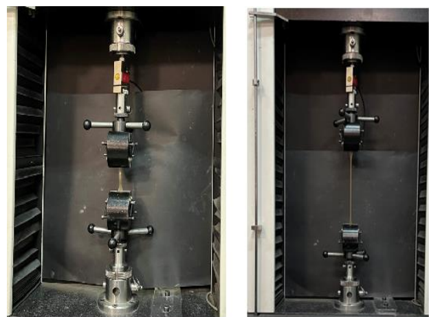
Fig. 2 Sample at the beginning of the tensile test (left) and during the tensile test (right)
