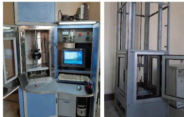
Fig. 2 Experimental apparatus of sandwich vein structures under a) quasi-static loading and b) low-velocity impact.
