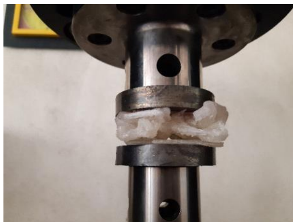
Fig. 6 Compressive tests for the bi-material lattice structure based on the quadrilateral bipyramid unit cell
