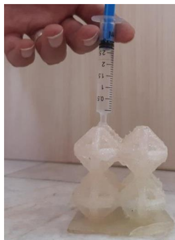
Fig. 5 Injection of resin into hollow struts
