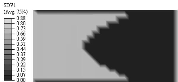
Fig. 8 Fatigue damage variable distribution in cohesive zone of sandwich panel after 70000 cycles for upper interface & core stiffness = 20MPa
