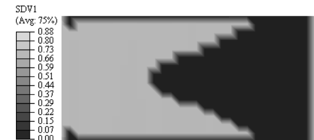
Fig. 9 Fatigue damage variable distribution in cohesive zone of sandwich panel after 70000 cycles for upper interface & core stiffness = 50MPa
