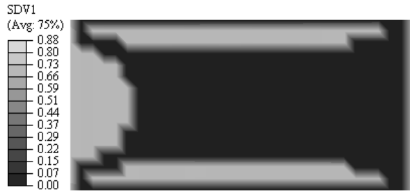
Fig. 10 Fatigue damage variable distribution in cohesive zone of sandwich panel for upper interface after 70000 cycles & core stiffness = 1GPa
