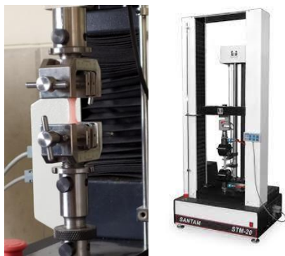
Fig. 1 Tensile test machine (STM-20)
