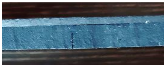
Fig. 6 Failure due to normal stress \sigma_x through the layers with fibers in 90^\circ direction in laminate with [90^\circ_3/0^\circ] stackup
