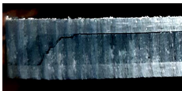
Fig. 12 Failure due to interlaminar shear stress through the layers with fibers in 90^\circ direction in [0^\circ/90^\circ_2/0^\circ] SFSF laminated plate under distributed load
