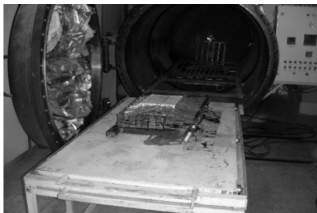
Fig. 2. Curing grid stiffened core in autoclave
