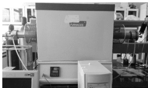
Fig. 3 Tubular vacuum furnace used in sintering process of specimens
